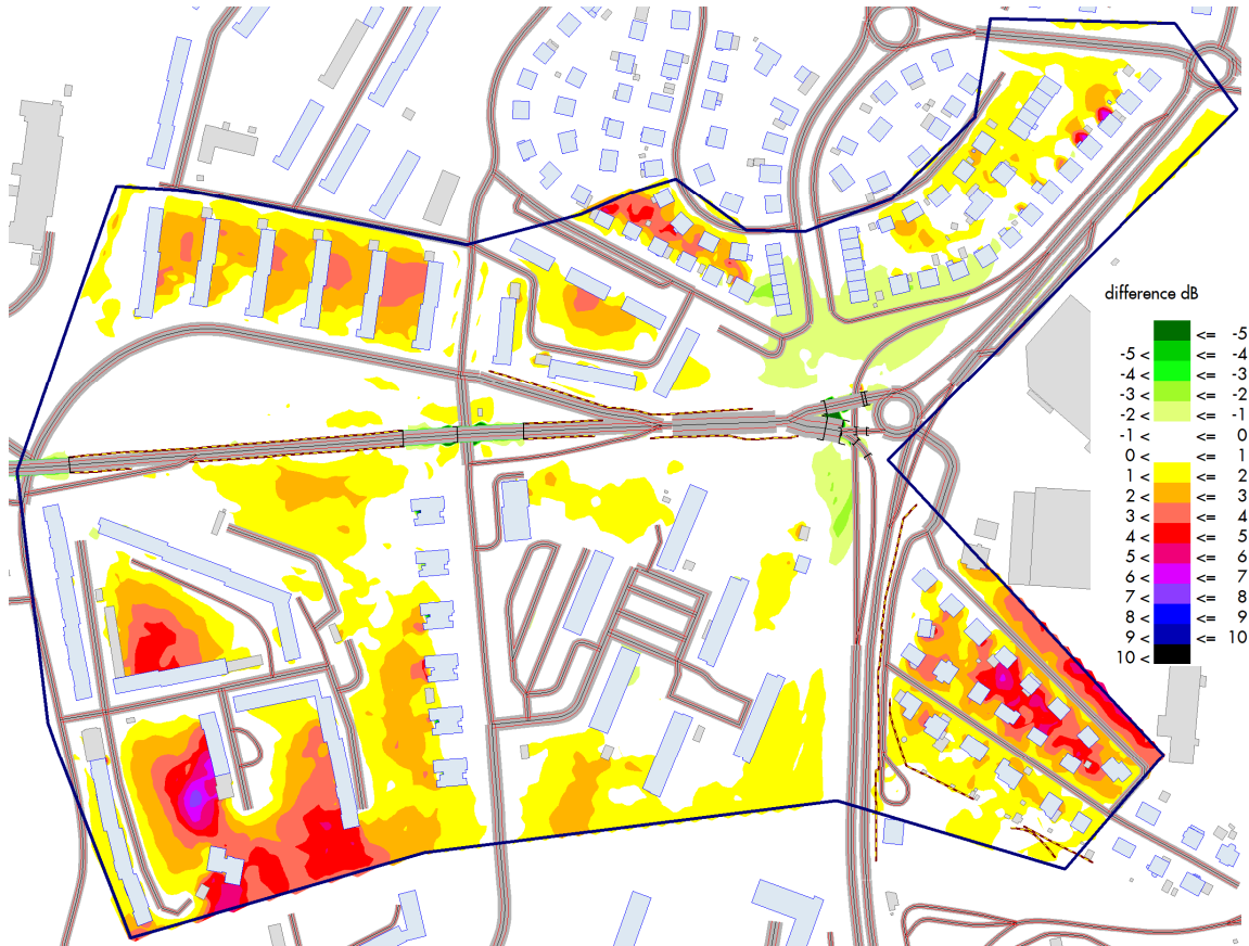
Figure 11: Differences between two noise contour calculations – a calculation made with Nord2000 using Danish weather statistics with four classes, minus a calculation with CNOSSOS-EU using default values of p_f . Arithmetic mean of all calculated points is +0.8 dB, median +0.7 dB, and standard deviation 1.5 dB. Noise protection walls are shown as black-yellow dashed lines.
